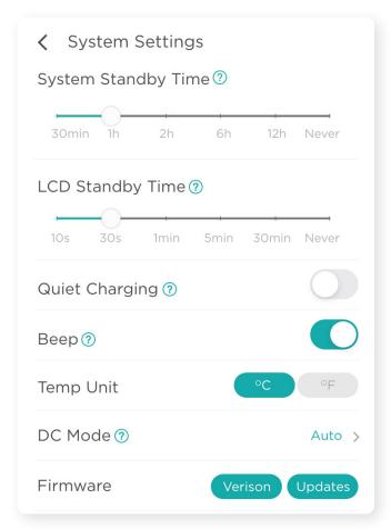
The system settings allow you to set the system standby time, screen standby time, silent charging, sound, temperature unit, DC input mode, view the device firmware version, firmware updates, restore factory settings, and more.
