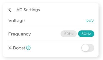
The AC power setting allows you to set AC output parameters, such as the AC output frequency (50Hz/60Hz).
