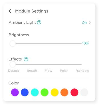
The module setting lets you adjust the parameters of different modules, such as the RIVER 600 MAX. You can adjust the switch, brightness, animation effect, and the color of the light.
